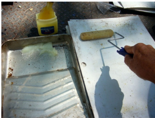
Applying petroleum jelly to sticky mat. Image courtesy The Food and Environment Research Agency (Fera), Crown Copyright.
